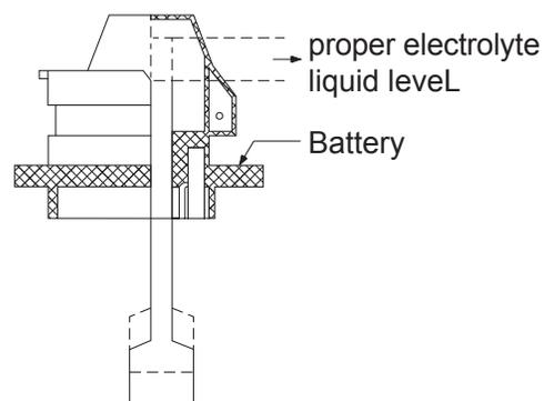
Add distilled water, red buoy will float until while rod appears under the red scale.
